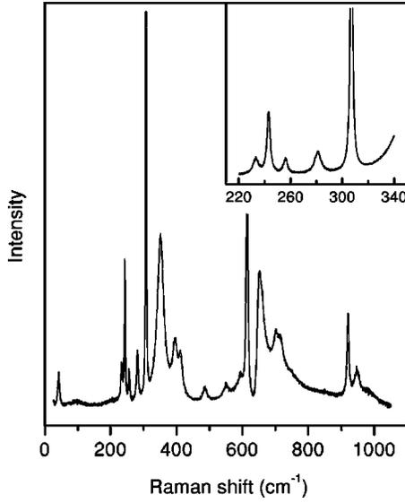
FIG. 1. Electronic Raman spectrum of Li-doped CdS measured with  $\lambda = 476.5$  nm at 4.2 K. The assignments of various peaks in the spectrum is listed in Table I. Inset shows the details of spectrum between the TO and the LO phonons. In order to focus attention on the weak modes, LO and 2LO phonons have been arbitrarily truncated.
