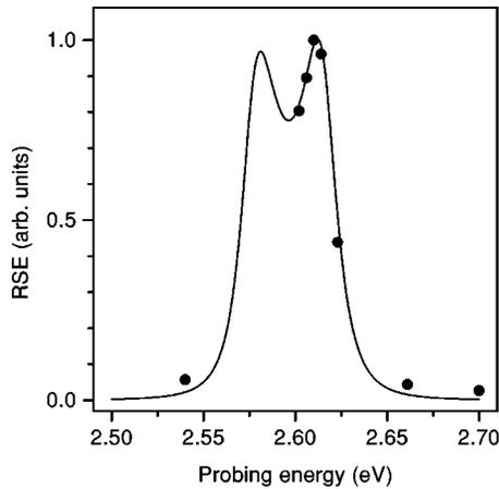
FIG. 3. Raman scattering efficiency of the LO-phonon sideband corresponding to the  $1s \rightarrow 2s$  hole transition. Full circles represent absolute experimental values and solid line shows a fit using Eq. (9), both of which are normalized to 1.
