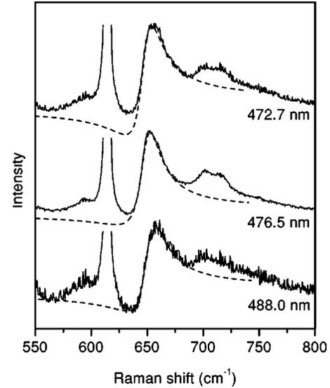
FIG. 2. LO-phonon sideband of the  $1s \rightarrow 2s$  electronic transition between bound-hole states of Li acceptors presented for three probing energies, which cover both sides of the resonance. Broken curves represent Fano-type fit using Eq. (2). In order to focus attention on the shape of the curves, the spectra are displayed at different scales.
