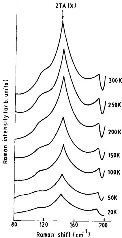
Fig. 5. Raman spectra showing the 2TA mode for ZnSe at various temperatures.
