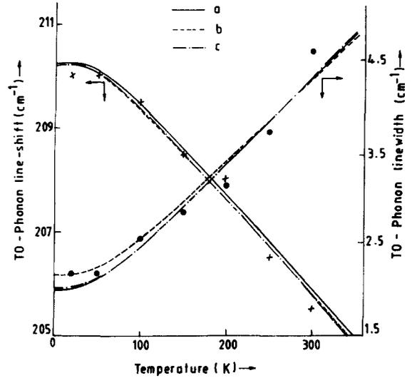
Fig. 2. Temperature variation in the line centre and line width for the one-phonon TO mode for ZnSe. The solid curves give theoretical fits using Eqs. (3) and (4), and the experimental points are shown by circles and crosses. The curves labelled (a)–(c) correspond to the decay processes labelled (a)–(c) in the text.
