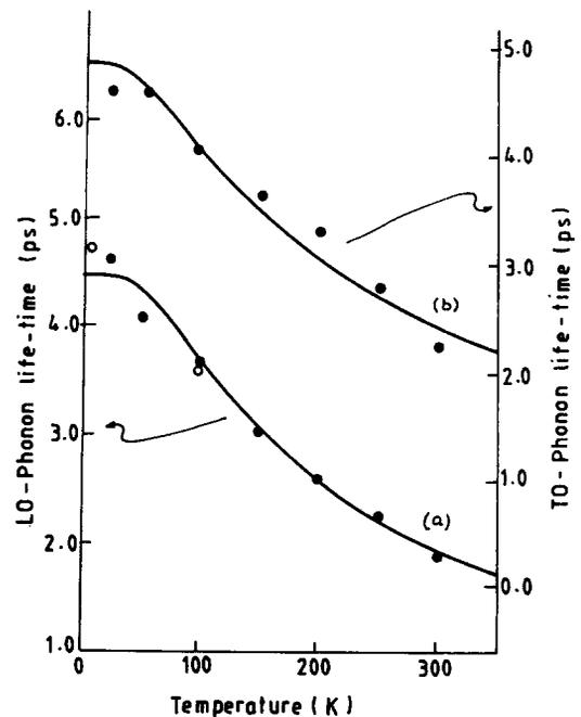
Fig. 4. Temperature variation in the phonon lifetime for (a) LO and (b) TO phonons. The solid curves show theoretical fits for the decay labelled (a) in the text, and the solid circles show our experimental results. The hollow circles are the values taken from Ref. [5].
