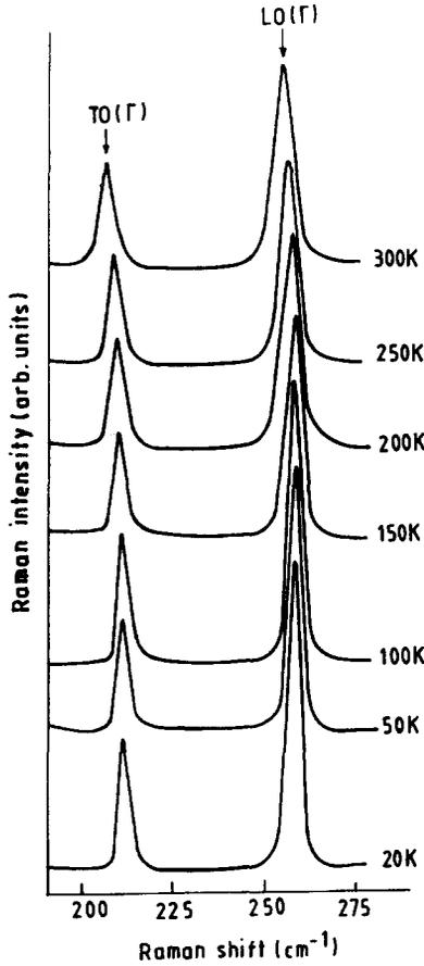
Fig. 1. Raman spectra of the <111> face of ZnSe at various temperatures showing the one-phonon optical modes.
