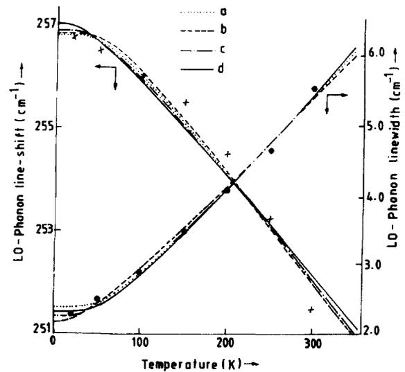
Fig. 3. Temperature variation in the line centre and line width for the one-phonon LO mode for ZnSe. The solid lines give theoretical fits using Eqs. (3) and (4), and the experimental points are shown by circles and crosses. The curves labelled (a)–(d) correspond to the decay processes labelled (a)–(d) in the text.
