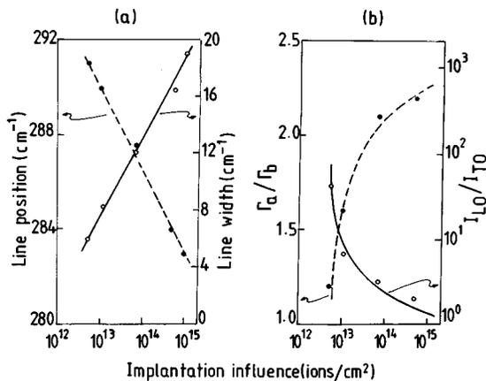
FIG. 5. Implantation fluence dependence of the line center and linewidth for LO-like phonon in P-implanted GaAs, (b) implantation fluence dependence of the asymmetry  $\Gamma_a/\Gamma_b$  and intensity ratio  $I_{LO}/I_{TO}$  for LO-like phonon in P-implanted GaAs.
