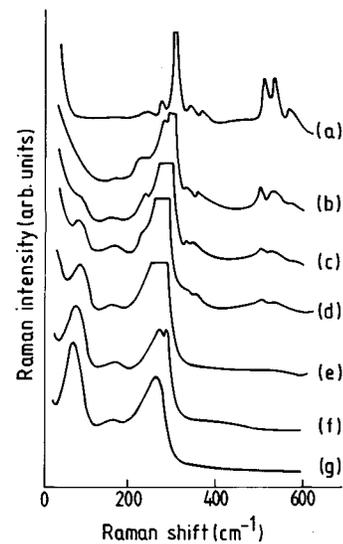
FIG. 2. Room temperature Raman spectra of P-implanted GaAs for implantation fluences (a) *c*-GaAs, (b)  $5 \times 10^{12}$ , (c)  $1 \times 10^{13}$ , (d)  $7 \times 10^{13}$ , (e)  $5 \times 10^{14}$ , (f)  $1 \times 10^{15}$ , and (g)  $5 \times 10^{15}$  ions/cm<sup>2</sup>.
