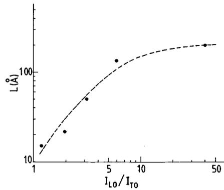
FIG. 6. The estimated values of the coherence length in ion-implanted GaAs for various observed values of the intensity ratio,  $I_{LO}/I_{TO}$ , in the Raman spectrum. The broken line is a guide line to the eye.
