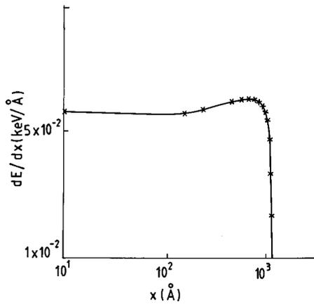
FIG. 1. Variation of the rate of energy loss of 70 keV P-ion in GaAs with distance from the surface.
