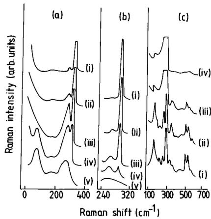
FIG. 7. Raman spectra of P-implanted GaAs at a dose of  $5 \times 10^{15}$  ions/cm<sup>2</sup> and subsequently PLA at various annealing power densities. Spectrum (i) in (a)–(c) correspond to the *c*-GaAs, spectrum (ii), (iii), and (iv) in (a)–(c) are for annealing power densities 20, 15, and 8 MW/cm<sup>2</sup>, respectively, and spectrum (v) in (a) and (b) are for *a*-GaAs.
