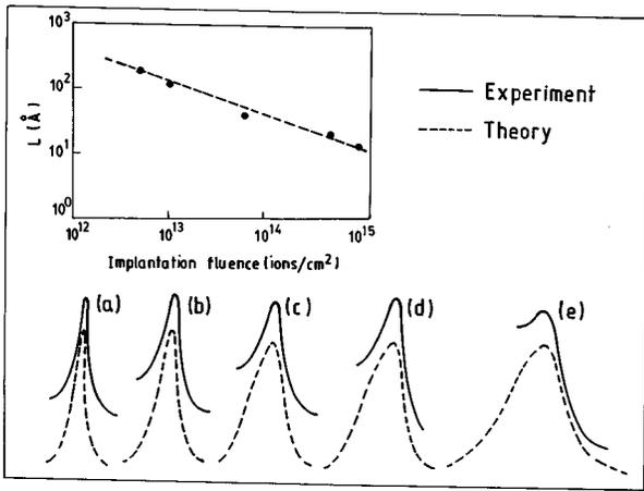
FIG. 4. Experimental and theoretical LO-phonon line shape for implantation fluence (a)  $5 \times 10^{12}$ , (b)  $1 \times 10^{13}$ , (c)  $7 \times 10^{13}$ , (d)  $5 \times 10^{14}$ , and (e)  $1 \times 10^{15}$  ions/cm<sup>2</sup>. The inset shows coherence lengths at various implantation fluences. The broken line in the inset is a guide line to the eye.
