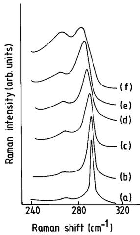
FIG. 3. One-phonon optical modes in the Raman spectra of P-implanted GaAs for implantation fluences (a) *c*-GaAs, (b)  $5 \times 10^{12}$ , (c)  $1 \times 10^{13}$ , (d)  $7 \times 10^{13}$ , (e)  $5 \times 10^{14}$ , and (f)  $1 \times 10^{15}$ .
