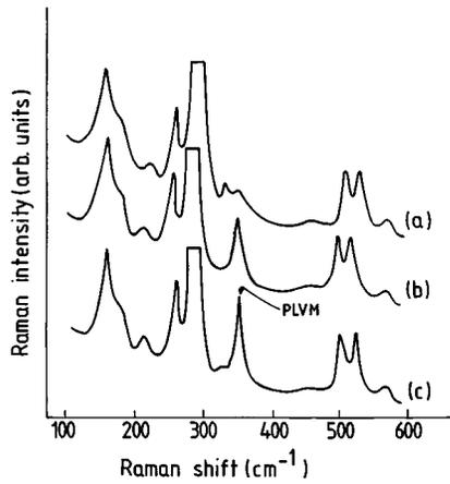
FIG. 9. Raman spectra of P-implanted and PLA GaAs showing the PLVM for implantation fluence (a)  $1 \times 10^{15}$ , (b)  $5 \times 10^{15}$ , and (c)  $1 \times 10^{16}$  ions/cm<sup>2</sup>.
