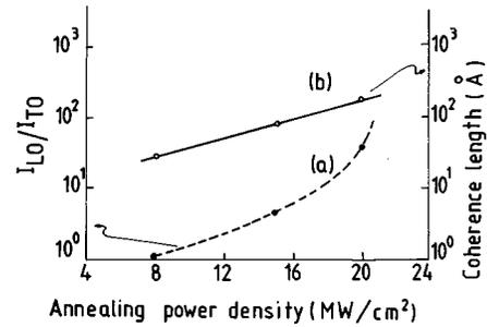
FIG. 8. The annealing power density dependence of (a) intensity ratio  $I_{LO}/I_{TO}$  and (b) coherence length in the PLA process of P-implanted GaAs.
