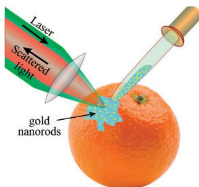
**Fig. 1.** Schematic illustration of PERRS experiment, where GNRs are spread over the outer surface of an orange to plasmonically enhance the resonant Raman signal from any pesticide molecules present on the surface of the orange.
