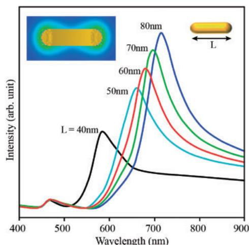
**Fig. 2.** Absorption spectra of GNRs with fixed diameter of 20 nm and various lengths from 40 to 80 nm, as numerically calculated using 3D-FDTD method. The left inset shows the locally enhanced electromagnetic near field for the laser excitation wavelength of 695 nm for an isolated GNR of length 70 nm.
