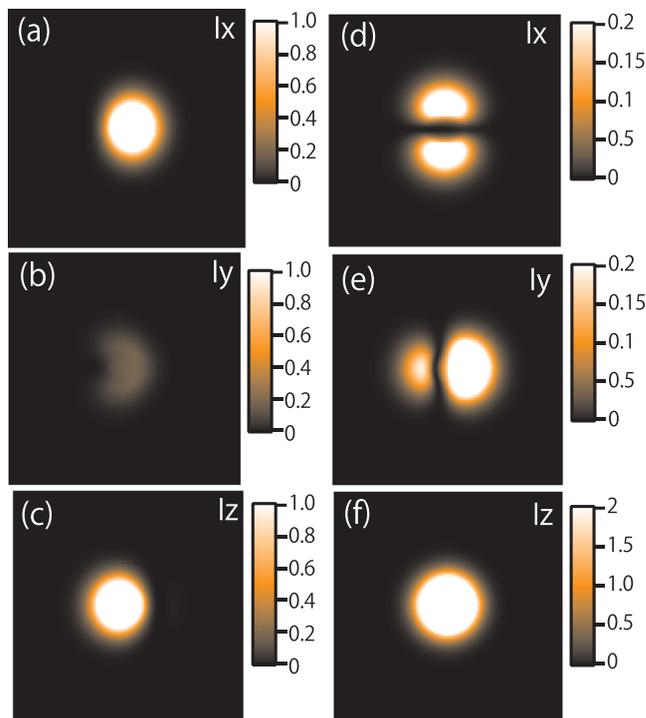
FIG. 3. Calculated near-field intensity and the spatial distribution of the polarization components  $I_x$ ,  $I_y$ , and  $I_z$ , generated by the  $x$ -dipole ((a), (b), and (c), respectively) and by the  $z$ -dipole ((d), (e), and (f), respectively) defined in Figs. 1(b) and 1(c). The calculation area was  $75 \text{ nm}^2$ .
