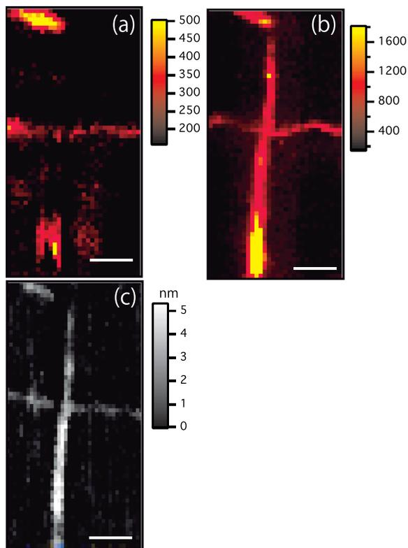
FIG. 2. TERS images of SWNTs (a) measured by the  $x$ -dipole and (b) the  $z$ -dipole. (c) AFM image of the corresponding area. The scale bars represent 200 nm.
