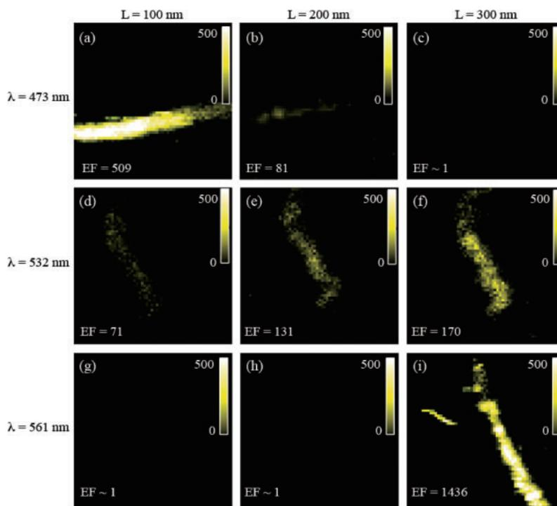
**Fig. 4.** TERS images ( $320 \times 320 \text{ nm}^2$ ) of CNT samples, constructed from the G-band intensity. The exposure time for each pixel was 0.5 s. The abbreviations EF, L, and  $\lambda$  indicate the enhancement factor, the length of the antenna, and the illumination wavelength, respectively.
