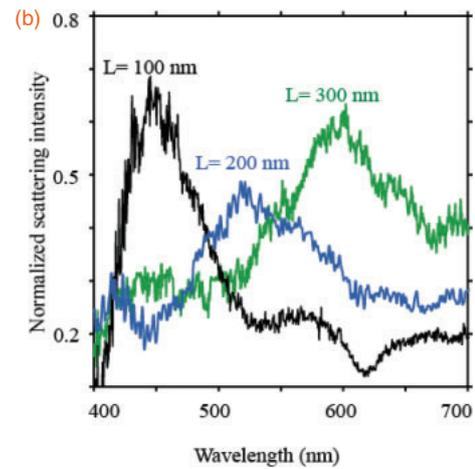
**Fig. 3.** (a) Schematic diagram of the experimental setup. (b) Scattering spectra of fabricated antennas with different lengths ( $L$ ).
