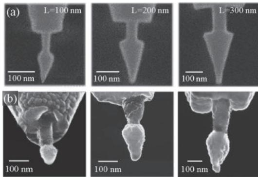
**Fig. 2.** (a) FIB images of FIB-milled AFM tips with different lengths, (b) SEM images of antennas with different lengths after the silver deposition.
