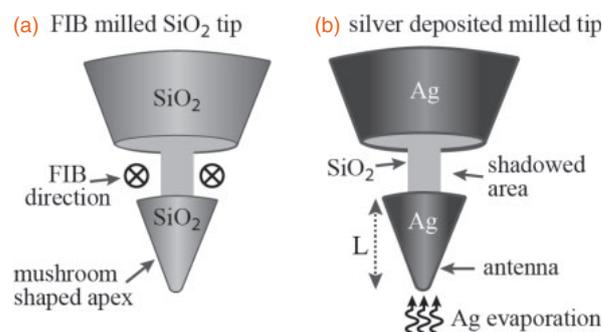
**Fig. 1.** (a) Illustration of FIB-milled ring shape on an AFM tip at distance  $L$  from the apex. (b) The mushroom-shaped apex can shadow the milled area during silver vapor deposition, and an antenna of length  $L$ , which is disconnected with the metal on the rest of the tip, can be formed at the tip apex.
