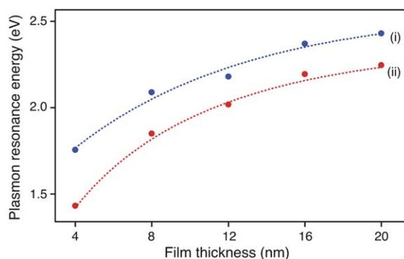
**Fig. 4** Energy of VS as a function of the film thickness in the gold tip–film system for tips with apex diameters (i) 15 and (ii) 30 nm. The dotted lines are the best fits obtained by using least square exponential curves to guide the eyes.
