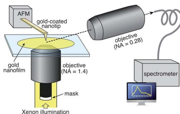
**Fig. 2** Schematic illustration of the optical setup for the measurement of scattering spectra for the gold nanoparticle–nanofilm system.
