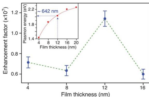
**Fig. 7** Enhancement factor in TERS measurement, where the sample was placed at the nanogap of a gold tip–film system, as a function of film thickness. The error bars represent the experimental error from 25 identical measurements. The inset displays the data for a 30 nm tip apex from Fig. 5 and shows that the VS plasmon energy for a film of 12 nm thickness matches the wavelength of the incident light,  $\lambda = 642$  nm.
