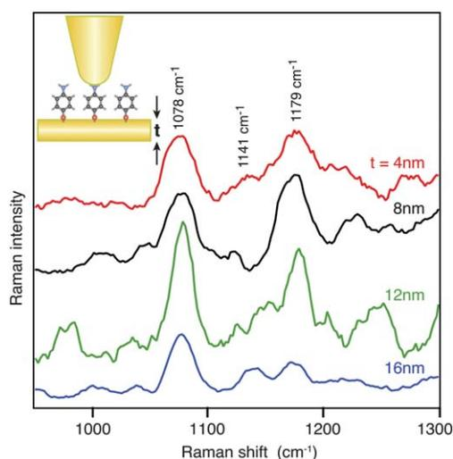
**Fig. 6** Tip-enhanced Raman spectra from a monolayer of 4-ATP molecules sandwiched between a gold-coated nanotip with the apex diameter of 30 nm and gold nanofilms with indicated thicknesses. The tip–film system, together with sandwiched sample molecules, is illustrated in the inset. The excitation wavelength is 642 nm.
