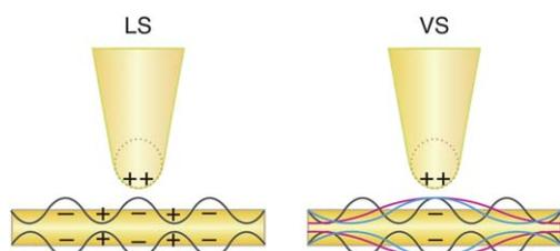
**Fig. 1** Schematic models of charge distributions for the LS (left) and VS (right) modes in a metallic nanoparticle–film system. The higher energy LS mode only couples efficiently to short wavelength film plasmons while the VS couples to longer wavelength film plasmons as illustrated by the three differently colored film plasmon modes.
