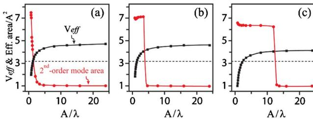
Fig. 2. (Color online) Effective  $V$  parameter (black squares and curves) and the second-order mode normalized area (red circles and curves) as a function of  $A/\lambda$  for (a) sixfold, (b) eightfold, and (c) tenfold quasi-crystal fibers. The dashed lines are drawn at  $\pi$ .
