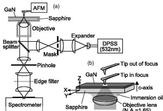
FIG. 1. (a) Schematic of the experimental setup for tip-enhanced Raman spectroscopy. (b) Enlarged view around focal area.
