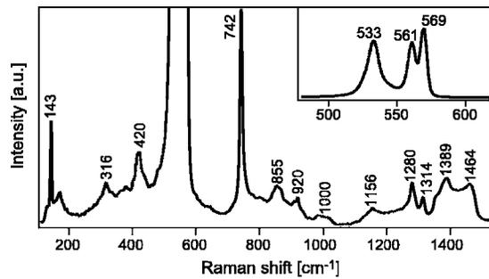
FIG. 2. Far-field micro-Raman spectrum of GaN, showing good crystalline quality.
