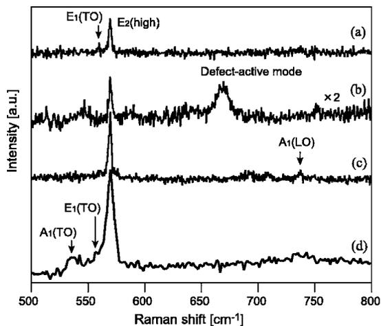
FIG. 4. Near-field subtraction spectra at some of the randomly chosen tip positions.
