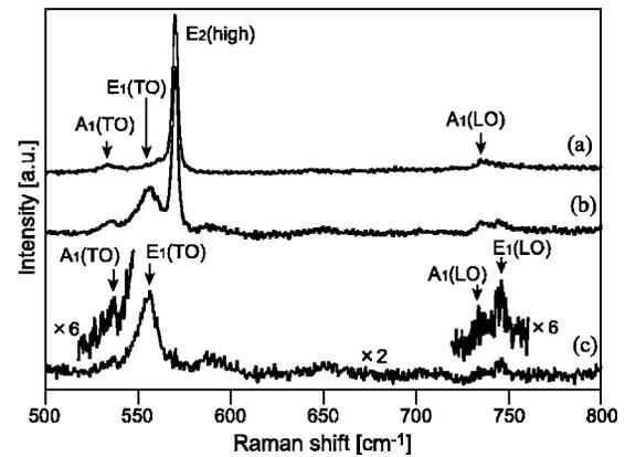
FIG. 3. Raman spectra obtained with tip (a) off the sample and (b) on the sample. The true near-field component obtained by subtracting (a) from (b) is shown in (c).
