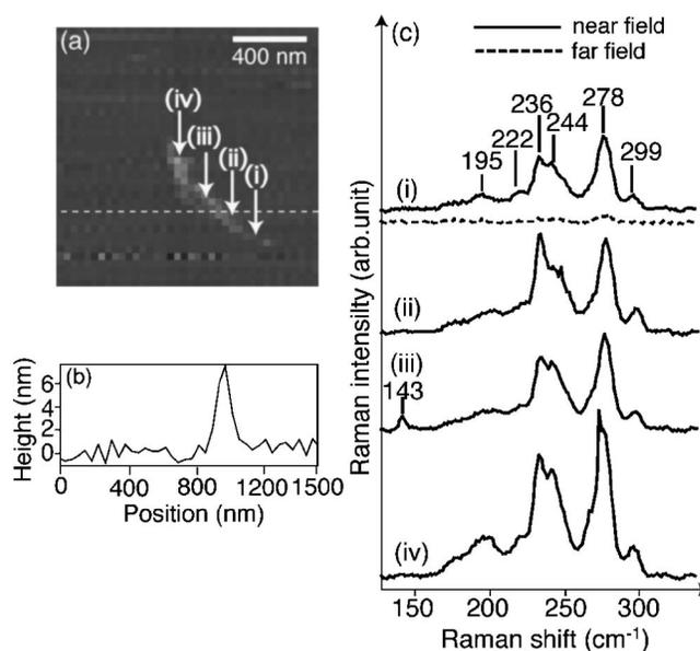
FIG. 1. (a) An AFM image of an individual SWNT bundle on the glass coverslip. (b) The line profile corresponding to the dashed line in the AFM image. (c) Tip-enhanced near-field Raman spectra measured over the bundle at the location indicated by (i)–(iv) in the AFM image.
