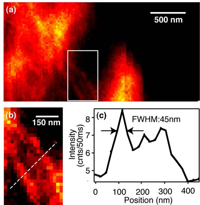
FIG. 2. (Color online) (a) Tip-enhanced near-field Raman image of SWNT bundles obtained at the frequency of 278  $\text{cm}^{-1}$ . (b) A zoomed view of a part of the near-field Raman image which is surrounded by the square in (a). (c) The Raman intensity line-profile depicted by the dashed line in (b).
