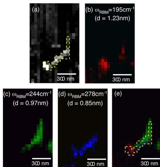
FIG. 3. (Color online) (a) An AFM image of a SWNT bundle. Tip-enhanced near-field Raman images were obtained at the frequencies (colors) of (b)  $195\text{ cm}^{-1}$ , (c)  $244\text{ cm}^{-1}$ , and (d)  $278\text{ cm}^{-1}$ . (e) The mixed color image obtained by combining the three images in (b), (c), and (d).
