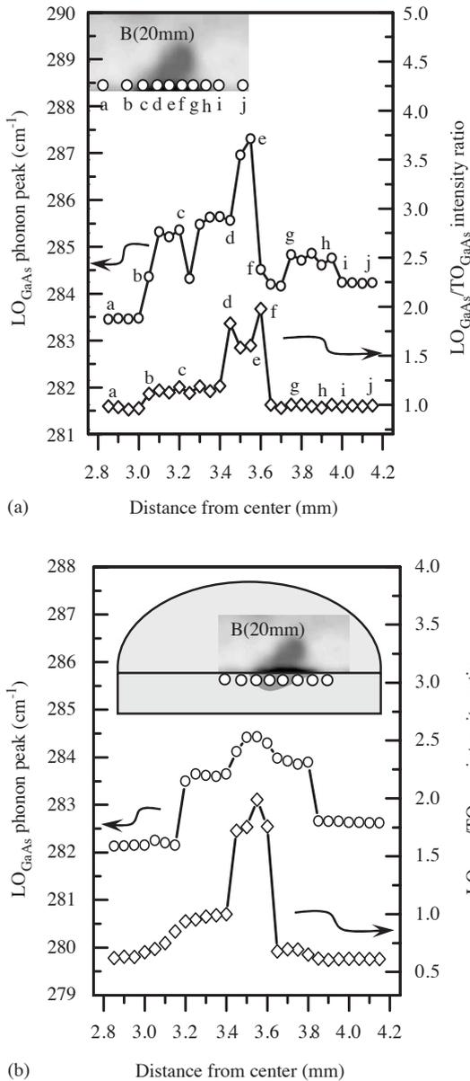
Fig. 3. (a) and (b)  $LO_{GaAs}$  phonon peak positions and  $LO_{GaAs}/TO_{GaAs}$  intensity ratio measured from the front and side surfaces of the wafer B, where left- and right-hand scales correspond to, respectively, phonon peak positions and relative intensity ratio. The insets show enlarged view of the investigated regions, in which open circles represent some of the measurement points.
