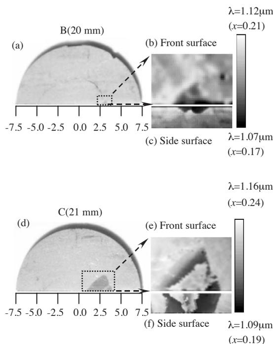
Fig. 4. 2D mapping images of PL peak wavelength measured in the wafers of B and C. The PL measurements were made in the region surrounded by dotted lines in the etching images of (a) and (d), also shown are those made at the corresponding side surfaces. The dotted lines and scales in millimeter represent the actual position of the investigated regions.
