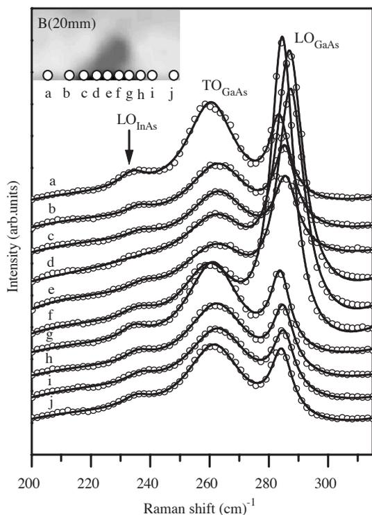
Fig. 2. Raman spectra measured near and in dark region from the front surface of the wafer B corresponding to the measurement points shown in the inset.
