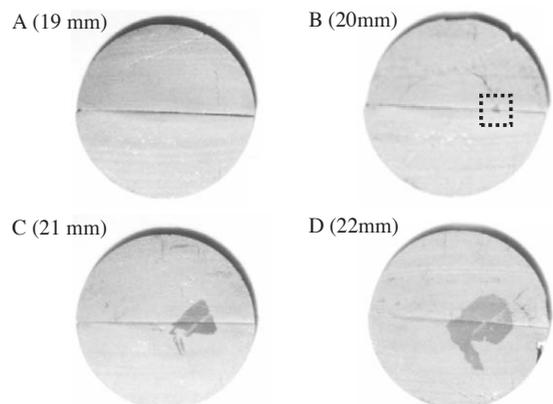
Fig. 1. Etching images of the wafers sliced at the different growth length of the crystal. A small black region shown inside the dotted square was found to increase in size with growth length. The crystallinity in this region appears to be changed with respect to the surrounding.
